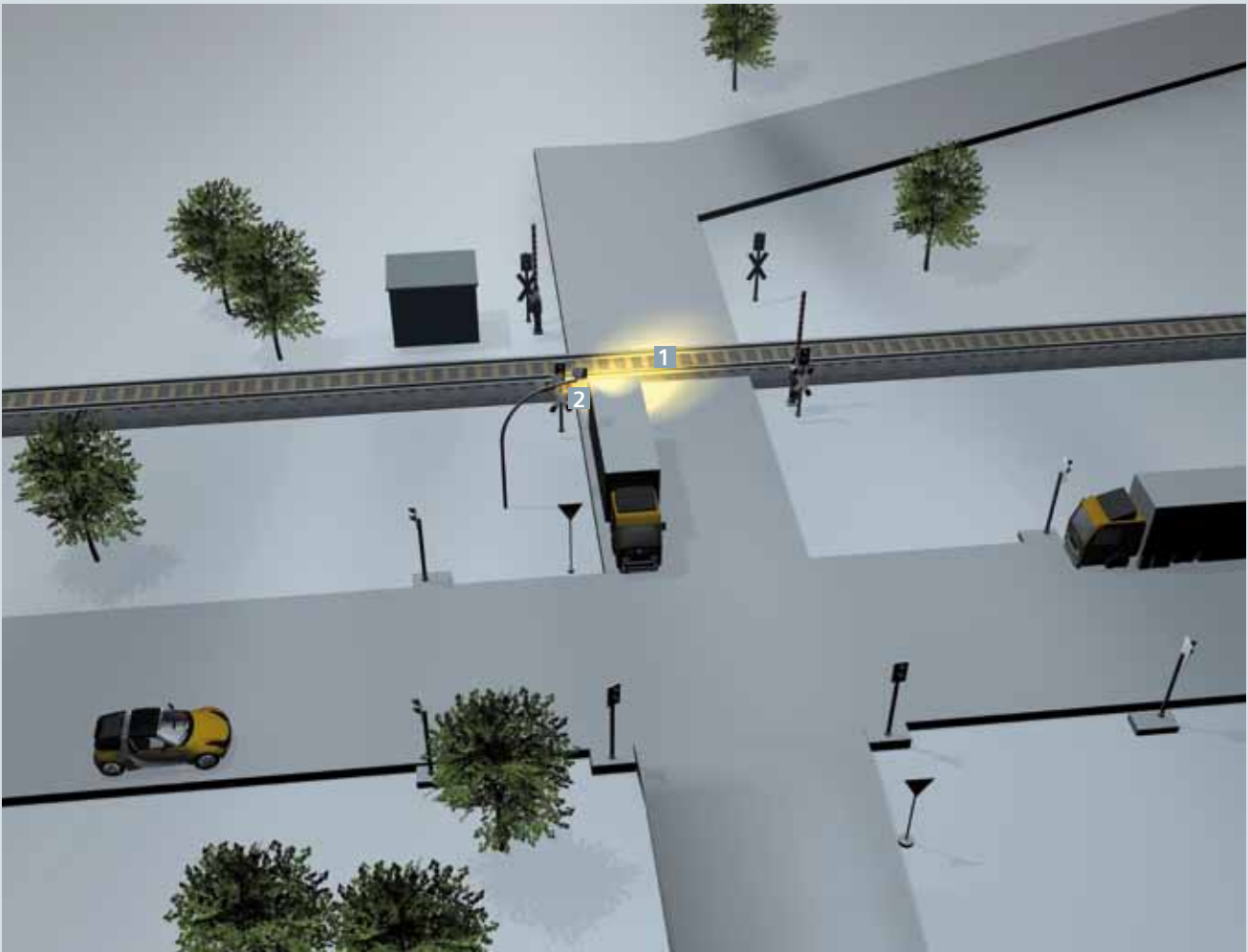
Road occupancy monitoring at a level crossing 1 Coverage of the danger zone by Siemens traffic detectors 2 A road traffic detector covers the danger zone
