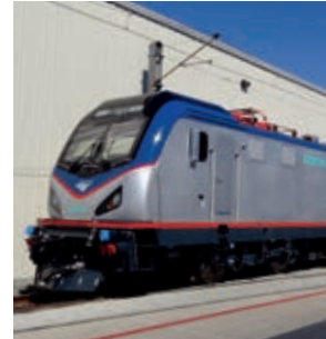
The Amtrak ACS64 can feed energy back into the grid while braking.
