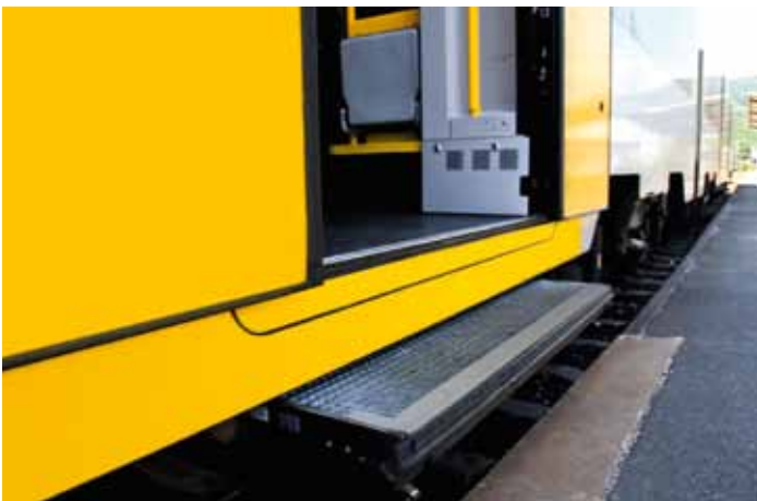
The step board helps passengers board and exit when platforms are low
