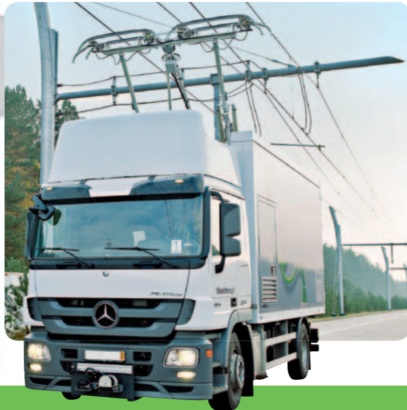
As with trolleybuses, e-trucks also require two contact wires.
