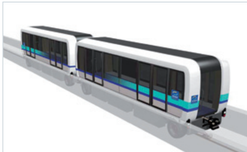
Val system in Rennes: driverless with 150-second headways.
