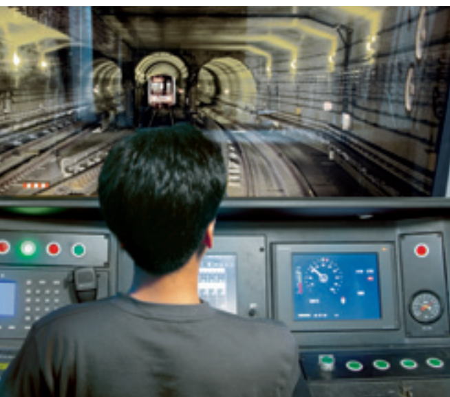
Line 10 of the Beijing Subway: ATO assists the driver.
