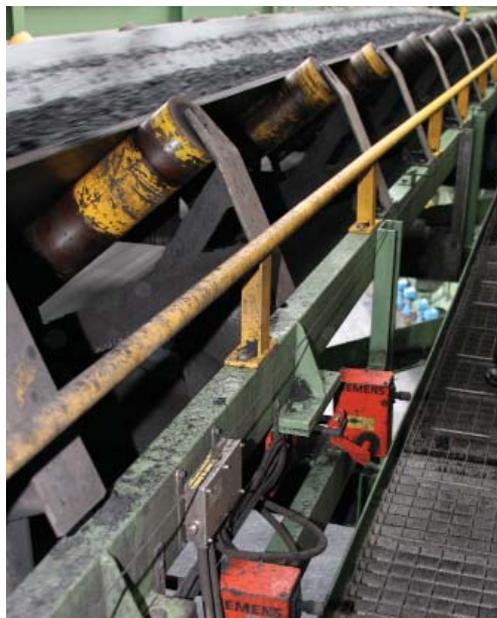
Siemens Milltronics MMI double-idler belt scale measures fast-moving coal on EMO's stacker-reclaimer.
