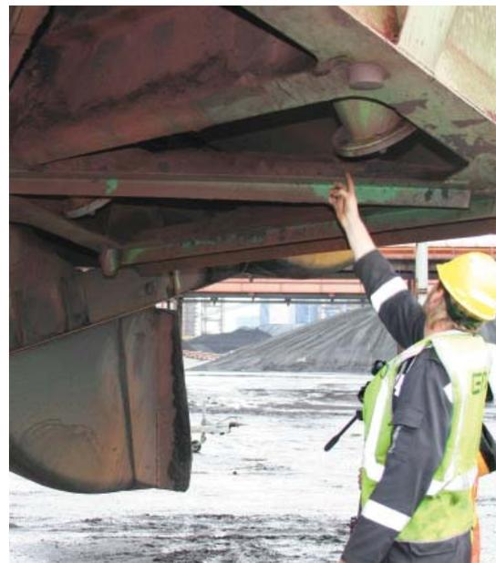
An EMO operator indicates the ultrasonic transducer located underneath the stacker-reclaimer's bucket wheel.
