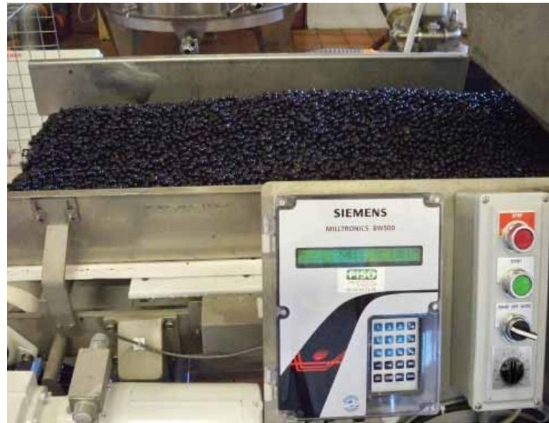
The Milltronics BW500 integrator determines and calculates the throughput quantities. The customer can now view yield details of individual appellations.
