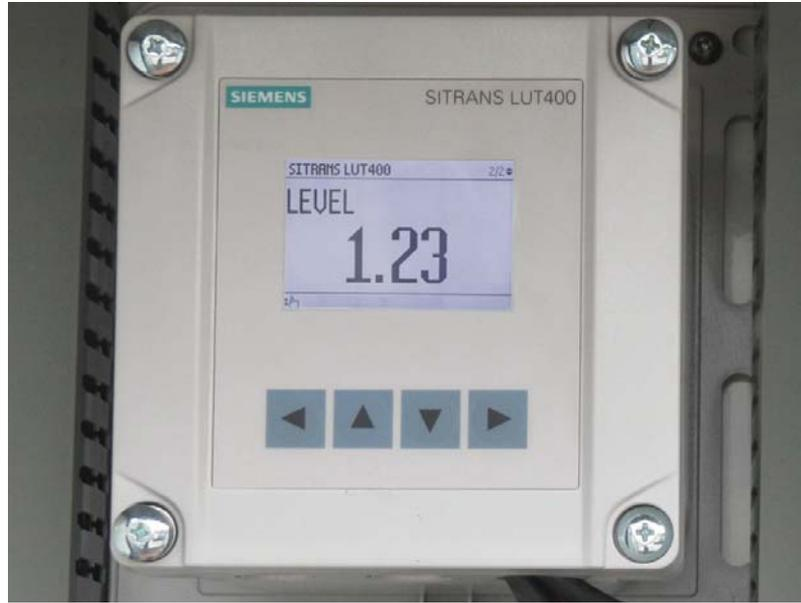
SITRANS LUT400 can be installed in a variety of mounting locations, including in panels, on DIN rails, pipes, or walls.
