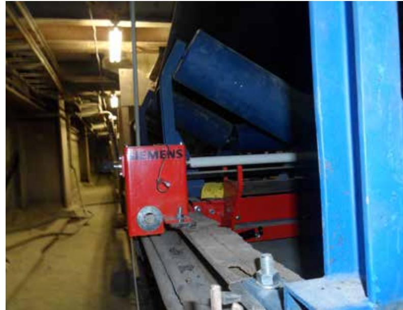
The Milltronics MWL weight lifter's modular construction, easily adapts to different conveyor widths including the large size 1400 and 1600 mm belts at Apatit.
