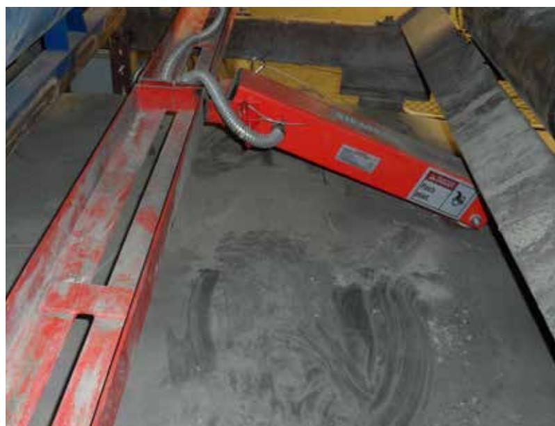
The rugged design of the Milltronics RBSS speed sensor is ideal for heavy duty applications. The RBSS offers easy, low cost installation while providing accurate belt speed detection
