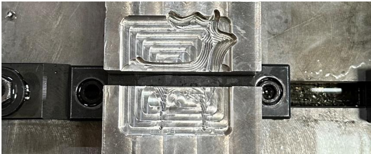
Clamping jaws for machining the rear side/clamping 2
