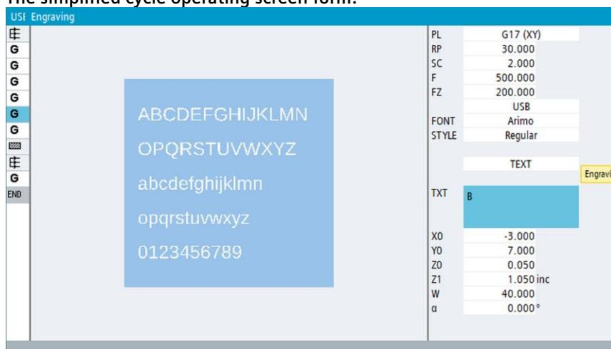
*Note: All entries in the cycle user interface must be completed using the Enter key so that they are applied in the NC program block and become effective. To edit the NC program, also at the PC, the key switch of the virtual CNC must be brought into position 3 (for Run MyVirtual Machine by clicking the mouse on the key switch icon on the user interface).*
