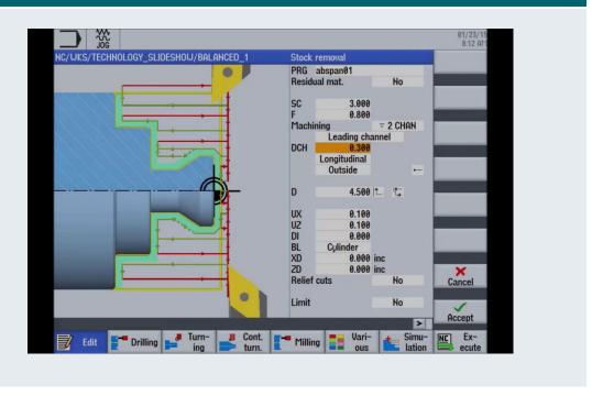
**Double the volume of metal removal** per unit of time can be achieved either by **doubling the feedrate** or by **doubling the effective infeed**. To do this, however, different strategies of tool path control are required.
