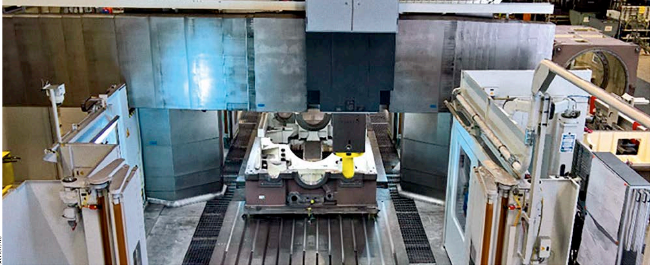
Machining workpieces weighing up to 40 tons on the MasterTec 3500 AT gantry milling machine equipped with a Sinumerik 840D sl CNC
