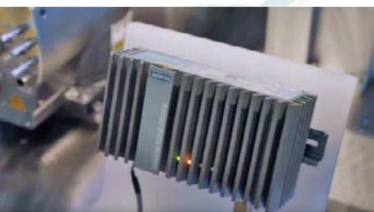
The Edge devices from Siemens are powerful and standardized industrial PCs
