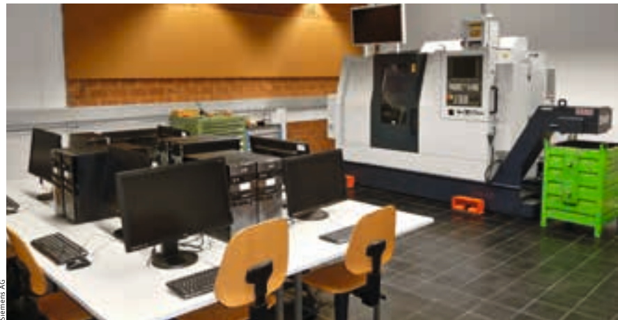
The classrooms are each equipped with a universal turning machine from Spinner with the Sinumerik 840D sl CNC
