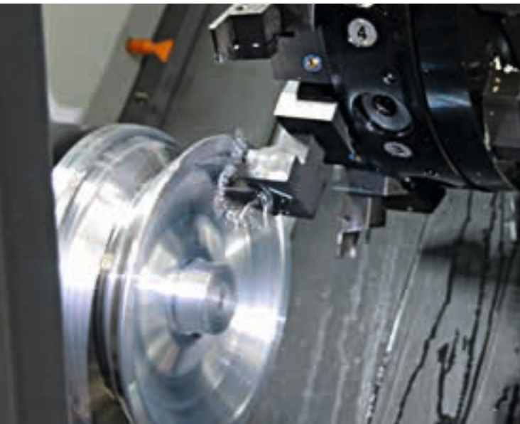
A special tool from Kennametal is used for plunge turning at Wirox, replacing several standard turning tools
