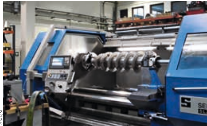
Machining a screw on a Seiger SLZ 1200E cycle turning machine with Sinumerik 840D sl
