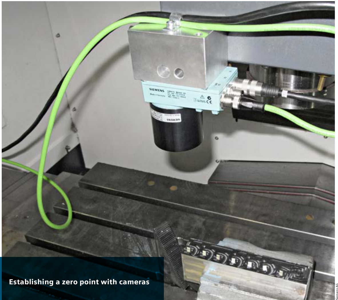
A Simatic MV440 1-D/2-D code-reader system in the machine space of a three-axis milling machine
