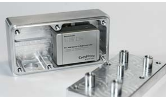
3-D simulation of the rear plate (above) and the finished milled camera housing (below)
