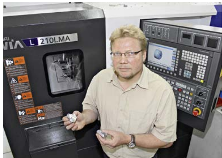
The new Hyundai L210LM turning center at Grenzmann can be retooled quickly thanks to the automatic clamping system, the automated calibration of the tools and the easy-to-use Sinumerik 828D CNC
