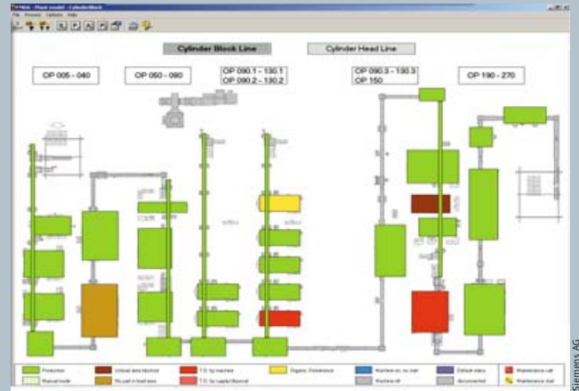
Example of a plant overview for a cylinder head and cylinder block line
