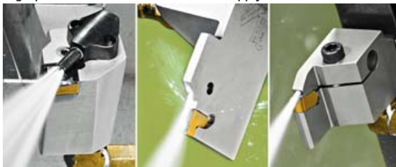
High-pressure tools with a controlled supply of coolant
