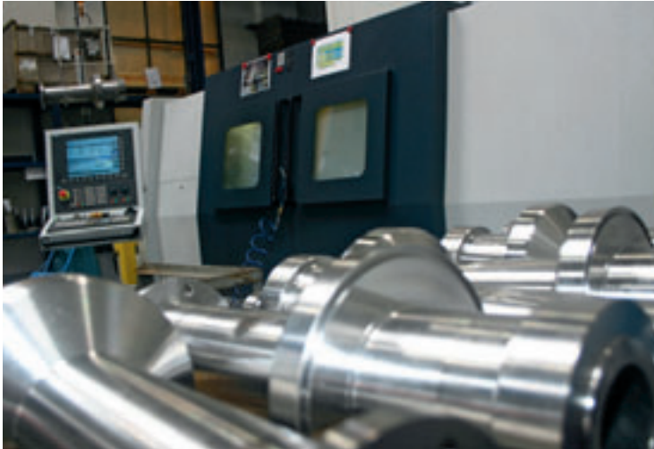
The Sinumerik-controlled Spinner turning machine with a subsequent finishing cycle ensures burnished, dimensionally accurate workpieces
