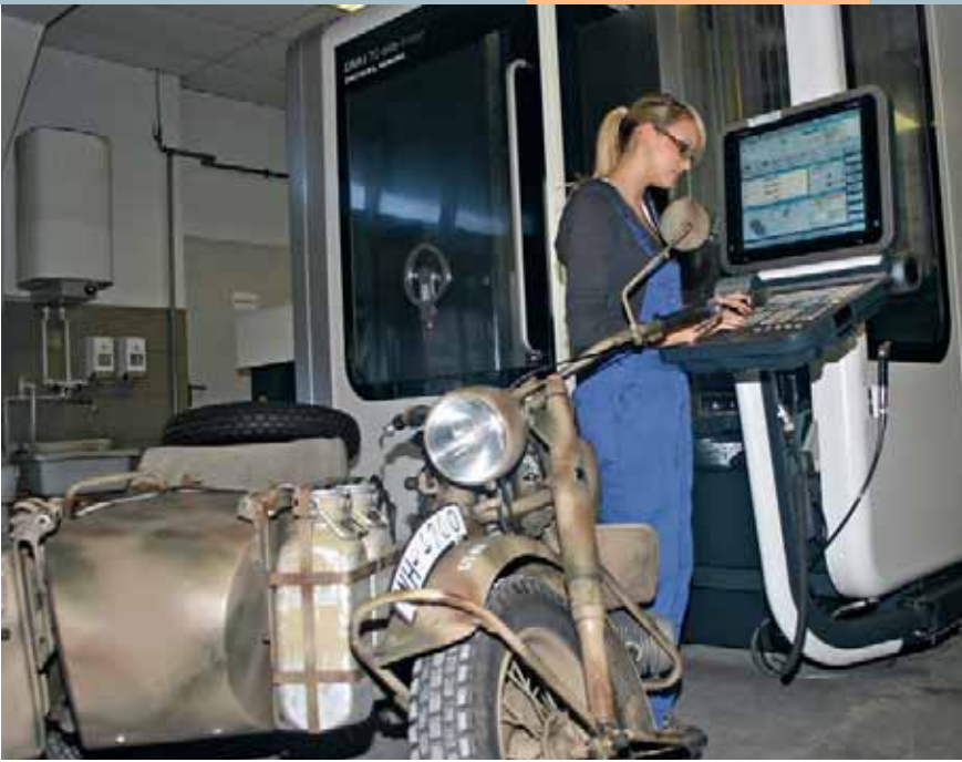
The skilled workers appreciate the easy menu navigation of the ShopMill programming interface when programming the special gearwheels
