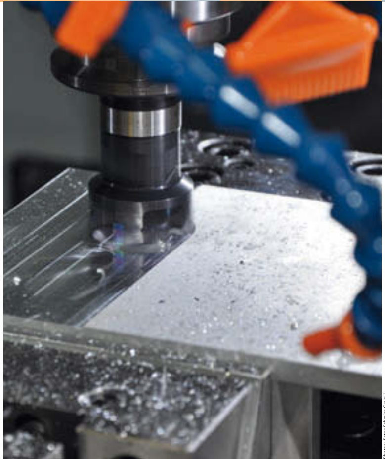
Face milling of a cooling pipe using the face milling cycle
