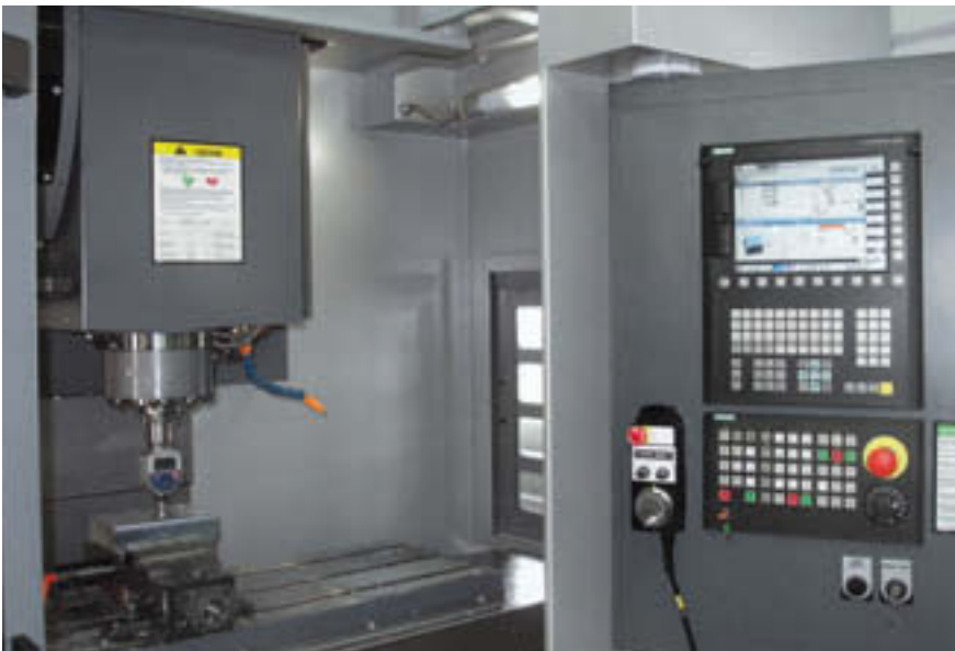
Animated graphics of the operating and programming software ShopMill support the user in setting up the milling machine quickly. Measuring probes determine the location of a workpiece in the machine and transfer the data to the controller. The Sinumerik 828D can then directly process the signals
