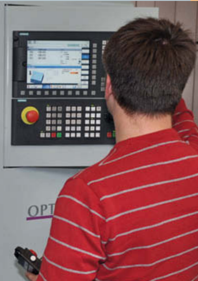
Zero point setup with mechanical measuring probes and the "Measure edge" cycle of Sinumerik Operate
