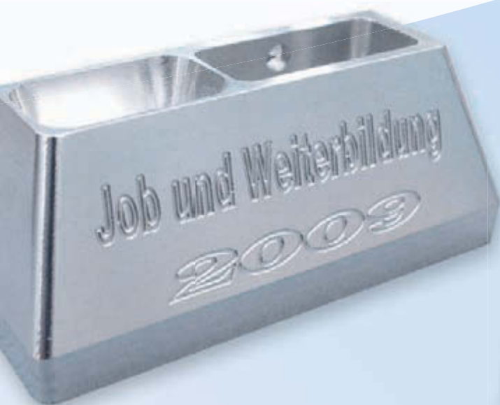
Milled complex parts with engravings or pockets made during various courses at the Chamber of Crafts
