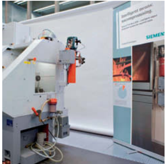
Fire protection on machine tools: a turning machine equipped with a Sinorix al-deco STD fire extinguisher at the TAC
