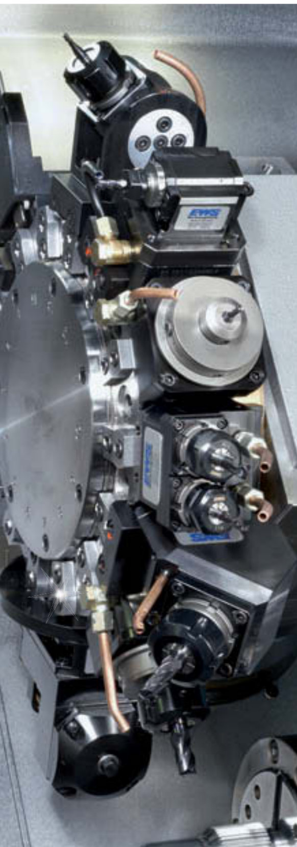
Multiple tool holders enable one work station to be equipped with several tools. "Simple" machines can be turned into machining cells that can process workpieces completely
