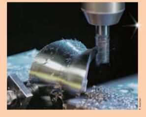
Implants for knee joints are precision machined with the HSC process of Sinumerik 840D sl
