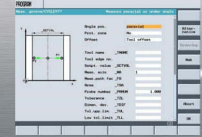
Automatic process measuring cycle: groove measurement with tool correction
