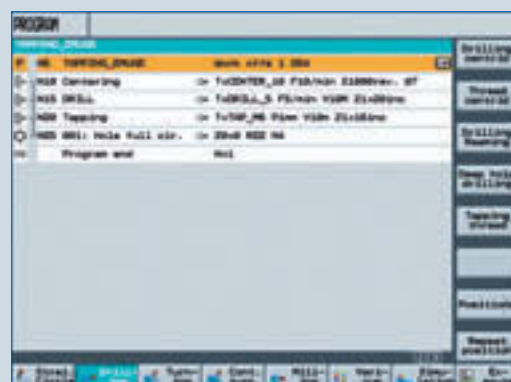
➔ Linked work schedule with hole circle position pattern for tapping
