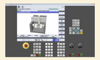
ith Sinutrain, Siemens offers users a perfect tool for the simple learning and professional training of CNC functions. The program works exactly like a real Sinumerik CNC. In the new software V4.5 ED.2, the collision avoidance function is now available in Sinutrain. This means
