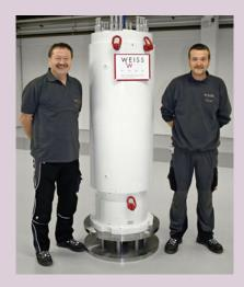
sion gearing. With about 80 kW of power, it is capable of producing 6,300 Nm of torque with a rotational speed of 120 min<sup>-1</sup> during continuous operation. During intermittent duty, it has a maximum torque of 8,350 Nm. These figures are especially important for manufacturing plants working in the aerospace, power generation and mining industries. The structure of the units is very similar to that of traditional motor spindles with powerful asynchronous
