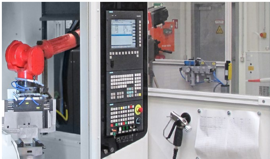
Full integration of robots within the CNC system simplifies robot-based machining of parts and the integration of CNC machines within flexible manufacturing networks
