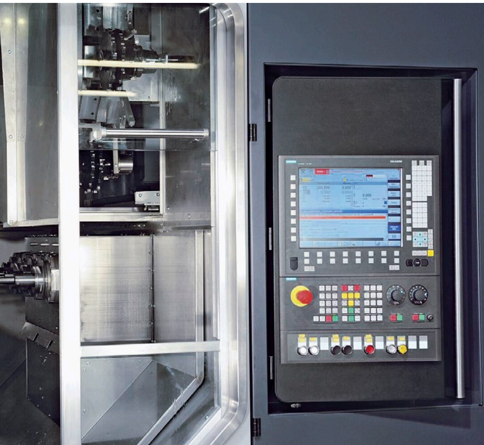
Fill uses the high-performance, flexible Sinumerik 840D sl type 1B CNC for machining demanding materials
