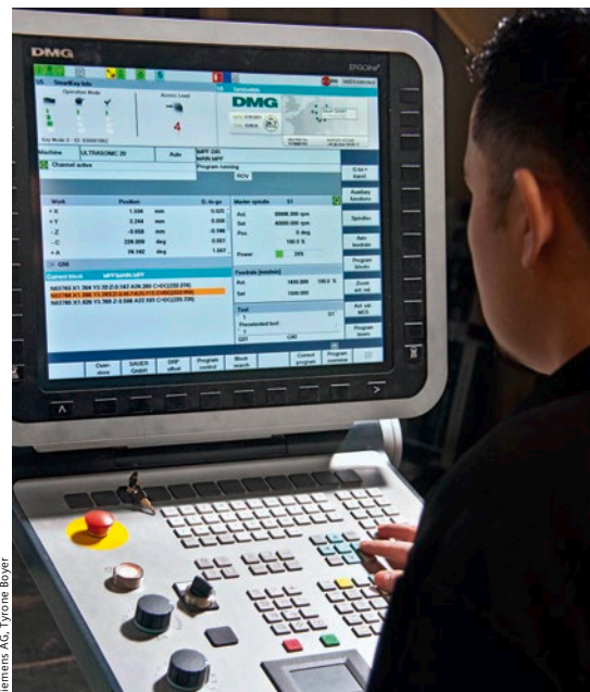
... and translates the cutting paths to the Sinumerik CNC
