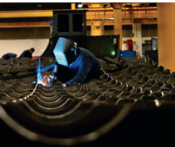
Coast Composites operates a complete metal fabricating shop, including metal bending and welding, in its Santa Ana plant. GTAW/GMAW welding is performed here
