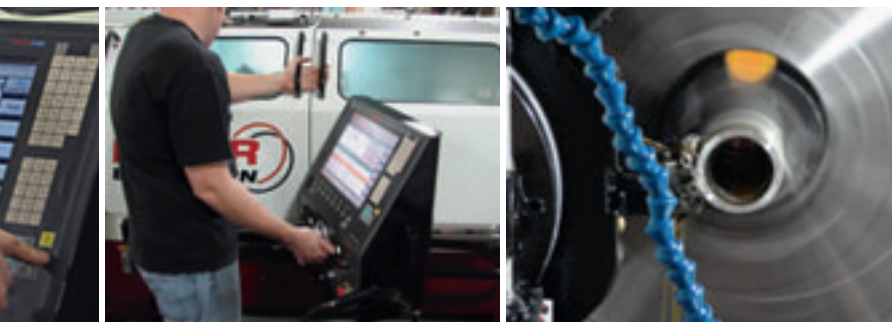
Siemens Sinumerik 840D sl CNC onboard the Fryer Easy Turn combination lathe
