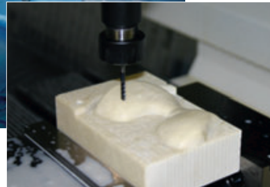
RenShape being machined on the DMG milling center
