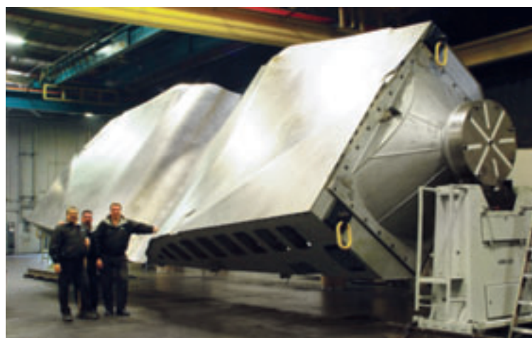
Coast Composites is a vertically-integrated supplier of Invar tooling, as well as mandrels and resin transfer molds used for composite layup in the manufacture of very large aerospace structures
