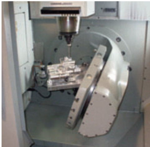
By adding a rotary table, a six-axis cutting theater was achieved
