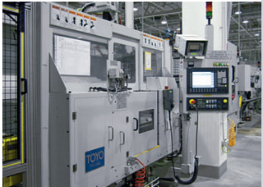
The CNC internal grinding machine is designed for mass production and equipped with a gantry loader as standard
