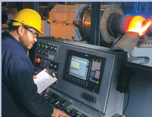
An induction heating system and shaping tools close the end of the steel tube for seamless integrity
