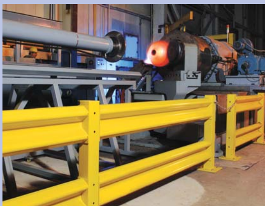
MJC's Model OSC-24300 at Fiba Technologies spins and forms tubes into pressure vessels over 40 feet long
