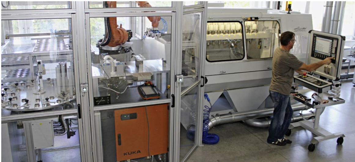
Thanks to Run MyRobot software interface, Silhouette production workers have no fear of using the robot. They can control it using the Sinumerik 840D sl operator panel, just like any other axis of the machine tool
