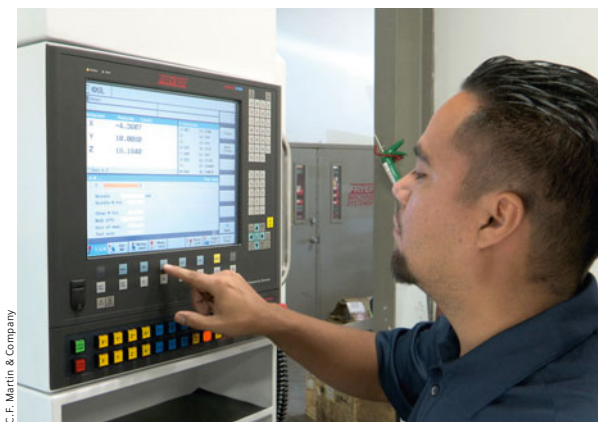
Left: Right-angle head compensation is essential to the accurate milling of guitar neck components. The function requires the sophisticated Sinumerik 840D sl CNC and ShopMill software from Siemens
