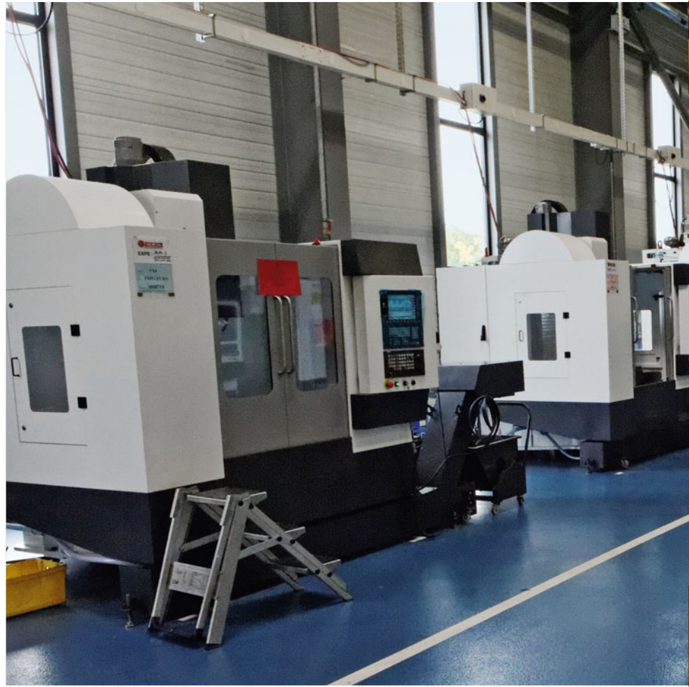
Huron equips its machine tools with Sinumerik CNCs and the Sinumerik Operate HMI system as standard
